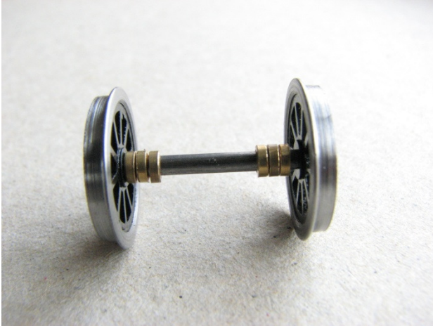
Bogie wheels assembled with spacing washers.
