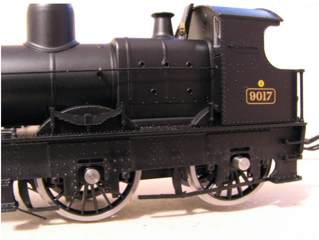
Keeper plate on and ready for the rods.
