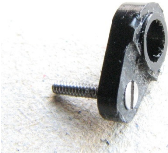
Outside cranks.... thinned slightly on the back.
