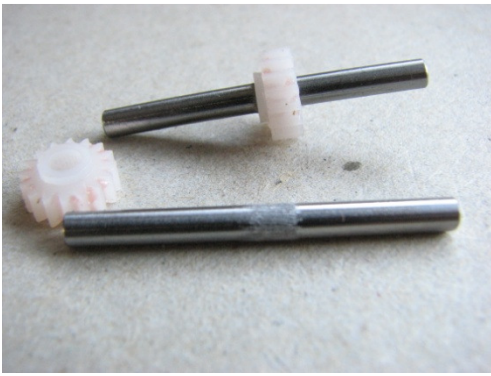
Gear on new axle – note boss faces chassis middle.
